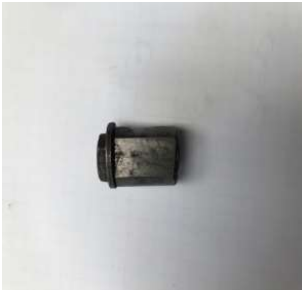
Camshaft follower brass guide remover Mk 1 Gudgeon Pin holder.
