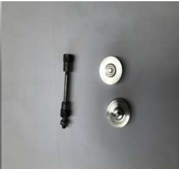
Camshaft follower brass guide remover Mk 1 Gudgeon Pin holder.
