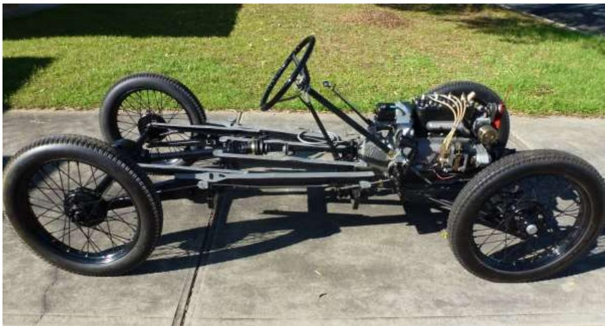
This has not happened in the last week. The car is a “build from scratch” project, starting with a bare chassis frame purchased from Club Spares in 1991. No point in rushing things. It has been fitted with the desirable 1926 magneto engine with a crack tested and reground 1-5/16” crank, new mains and big ends, uprated oil pump, alloy sump, Repco-modified camshaft and an Ulster cylinder head. The gearbox features close ratio 3-speed gears from Club Spares, new bearings and seals.
